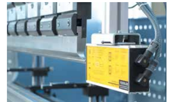
Ce Laser Safety System
