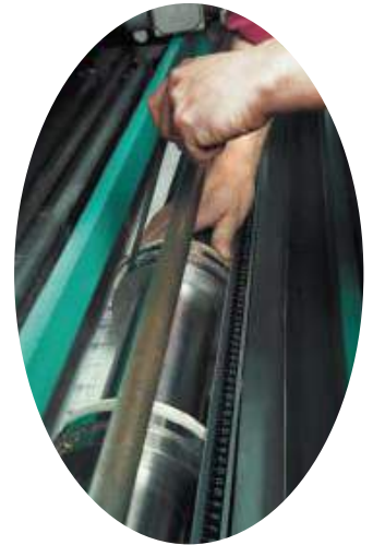
easy access and fast adjustment of the blades
