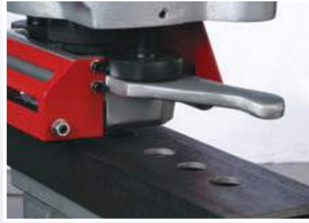
Punching channel flanges and angles
