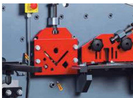
In this station standard rectangular notching and with special blade triangular notching can be performed
