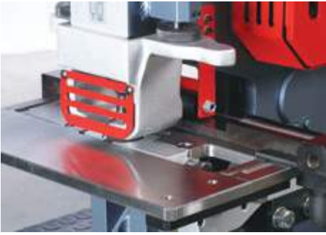
Punching station has max. Capacity of 27x13 & 18x18
