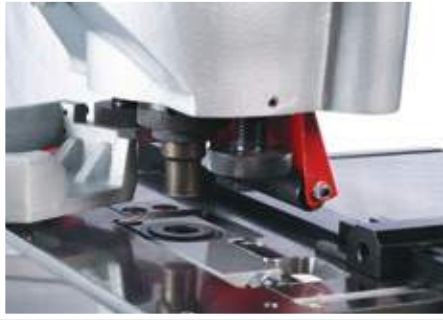
The punching station comes standard with quick change punch and die holders, as well as a swing away stripper
