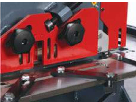
This station allows to cut special bars with special blades such as round, square, channels and many other special profiles
