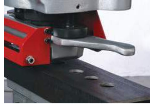
Punching Channel Flangers And Angles
